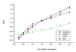
Fig. 2: Photometric titration curves of: TMP-I<sub>2</sub>, TMP-DDQ, TMP-CHL and TMP-PA reaction in CHCl<sub>3</sub>.
