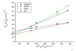
Fig. 3: The plot of  $C_a{}^o(4C_d{}^o+C_a{}^o)$  against  $C_d{}^o.C_a{}^o{}^2/A$  of: TMP-I<sub>2</sub>, TMP-DDQ, TMP-CHL and TMP-PA reaction in CHCl<sub>3</sub>.
